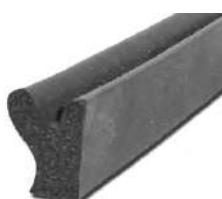
Extruded "V" shape foam for all 1963-74 models seals the trunk lid preventing water leaks. Please measure original seal for correct footage when ordering.
