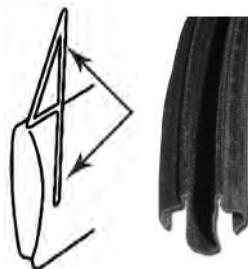
U-shaped strip that fits on the backside of the vent window channel where the door window rolls up into.
