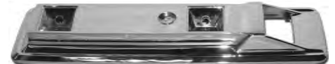
1968-70 B-Body reproduction 13" front armrest bases. These bases feature the correct smooth chrome finish and accept 9 1/2" armrest pads.
