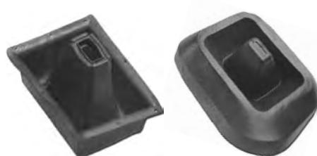
Shifter boots made for 1970-72 models with a console and standard transmission. Upper boot fits on top of the console and is molded to accept the shift ornament while the lower boot fits under the console on the floor board.
