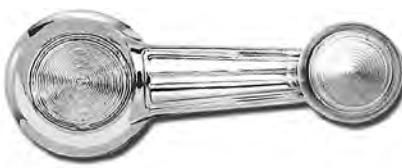
Die-cast reproduction of the original chrome front and rear window crank handle for all 1967-72 models.
