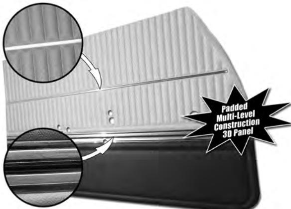
This Legendary product features as-original Die-electrically heat sealed Double Diamond grain upper section with Madrid grain lower section and chrome accent strip. Special cutout area in filler board to accommodate armrest base. Padded Multi-Level Construction 3-Dimensional Panel.
